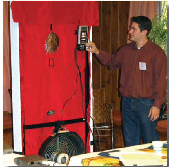
As shown in this demonstration, a blower door can be fitted into the doorway of a home and depressurizes the home to detect the places where heated or air-conditioned air is escaping from the home.
